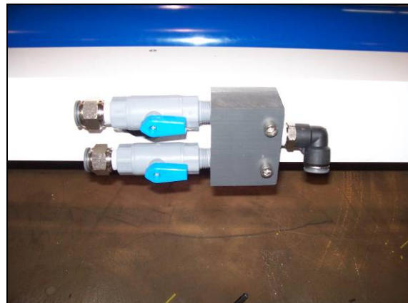
Picture #7 Water Manifold Mounted
